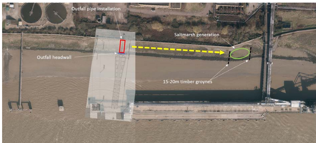
Figure 3 – Indicative location/layout of Thames outfall culvert, headwall and scour protection apron (image overlain on west/left); and indicative location/layout of proposed saltmarsh mitigation comprising groyne within area targeted for saltmarsh generation (green ellipse shown to east/right).
